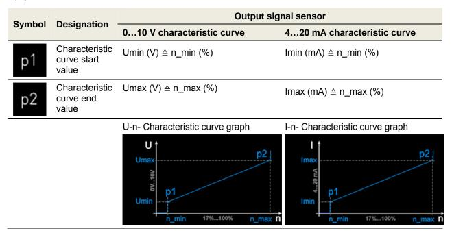
Tab. 11: Parameterization automatic sensor
