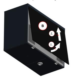
Fig 12: Opening the front plate
