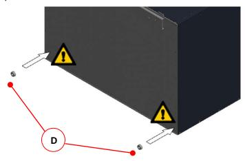
Fig 19: Mounting of the rubber puffer
