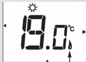
Radiator heating indicator
