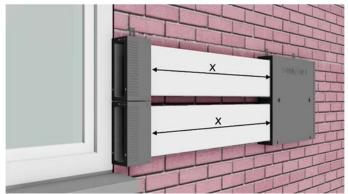
6. First attach the inner U-channels of the flat duct insulation by pushing them in between the shell wall and the flat duct (6) from above or below. Then clip the outer U-channels of the flat duct insulation onto the inner U-channels using the tongue and groove system.
