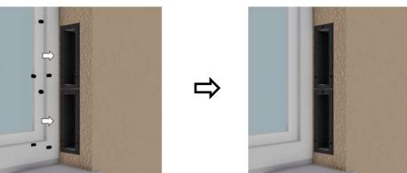
2. Place the discharge grilles (10) on the duct adapters (8) and fasten them in place with the M5x16 countersunk screws supplied.
